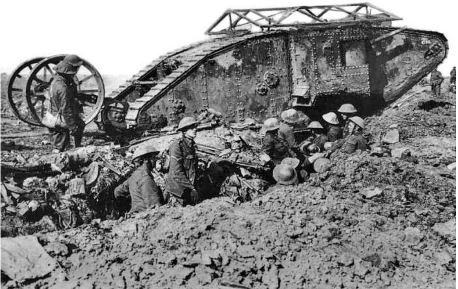
A Mark I tank, moving from left to right. The rhomboidal shape allowed it to climb parapets and cross trenches. Photo by Ernest Brooks
